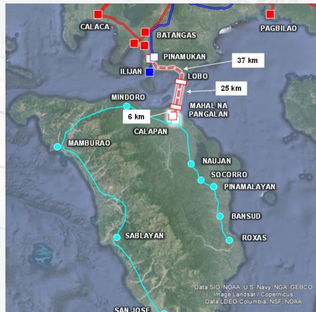
Figure 11.3: Batangas–Mindoro Interconnection Project
