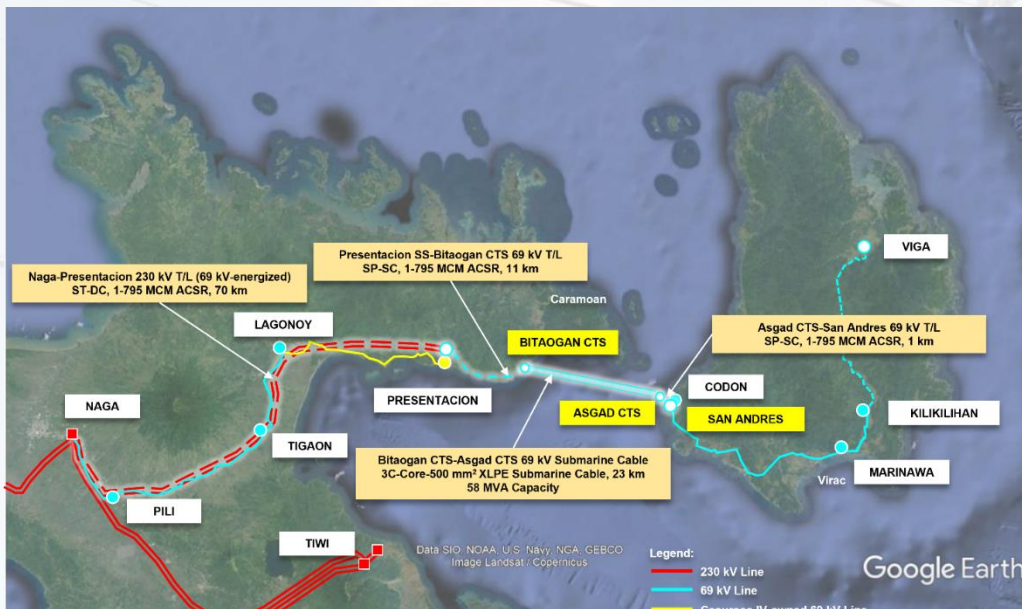
Figure 11.11: Camarines Sur – Catanduanes Interconnection Project
